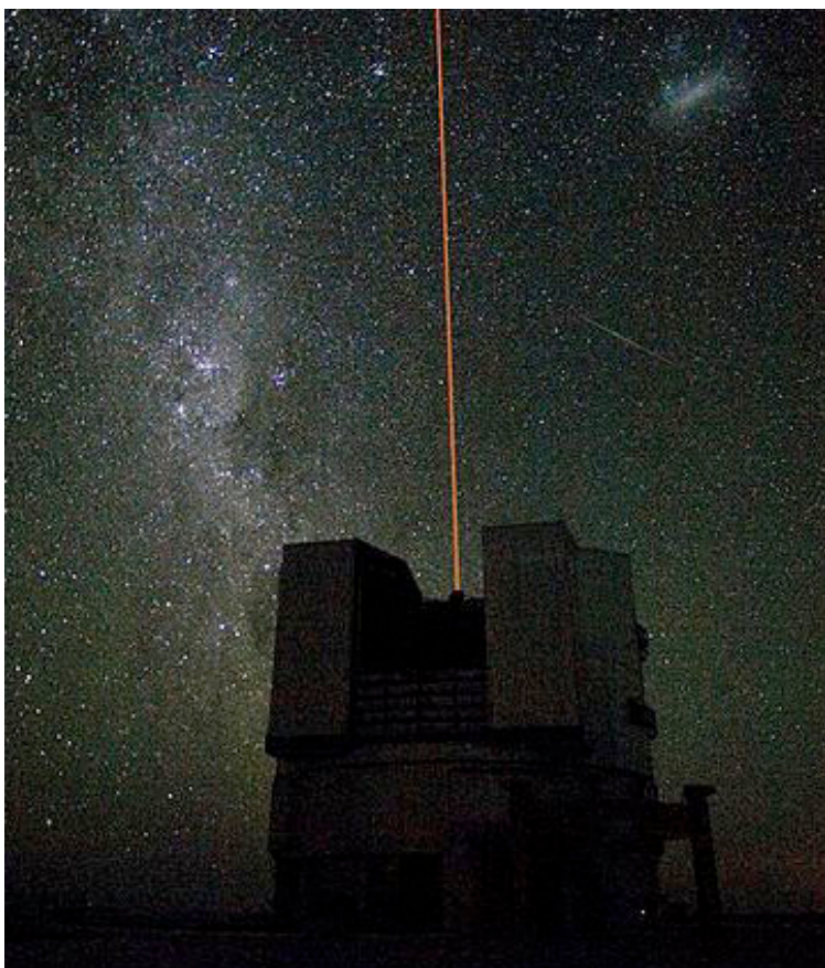
Figure 2. Much higher power lasers are used by professional astronomers to provide artificial guide stars for adaptive optics systems on large telescopes. Here a beam is projected from one of the 'unit telescopes' of the ESO Very Large Telescope (VLT).
