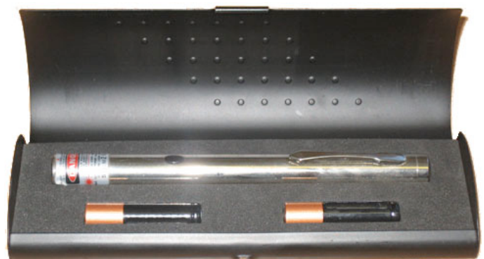
Figure 1. A typical hand held, battery operated laser pointer, shown in its case with batteries. The labelling on the laser should include the maximum power.
