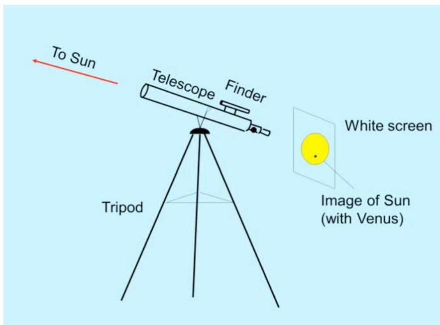
Figure 3 – How to project an image of the Sun through a telescope.
